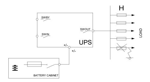
In order to select the correct protection devices to be inserted downstream of the LIBRAPRO PF1, the following two operating modes have to be taken into consideration: *mains power supply* and *battery power supply*.
