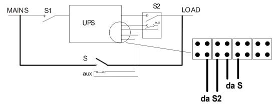
Additional output disconnector S2, additional disconnector S of the external maintenance by-pass. The auxiliary contacts S2 and S must be connected to terminals P and Q.
