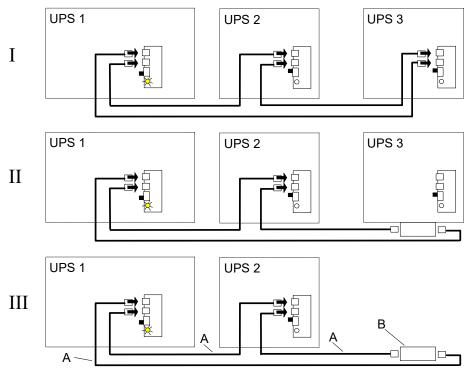
A)UPS parallel cable type RJ45
