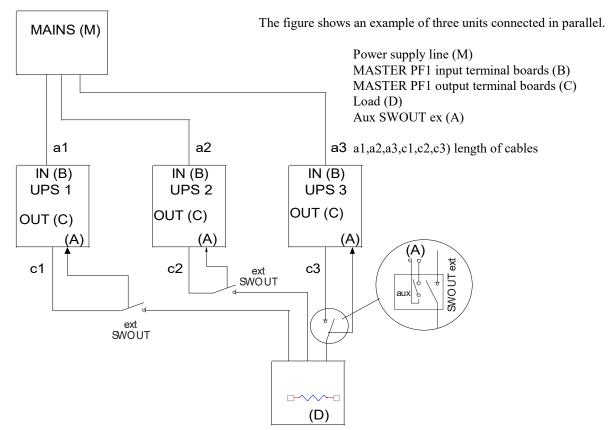
NOTE: "SWOUT ext" must be provided with an auxiliary contact (open with the switch open and closed with the switch closed).
