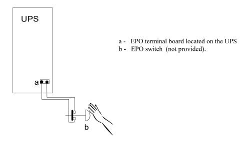
On the LIBRAPRO PF1, the jumper on the EPO terminals (page 20) must be removed, and the wires from the auxiliary contact of the button must be connected in place of the jumper.
