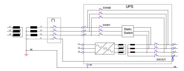
NOTE (\*): place the label supplied (*The following label, supplied with the UPS, must be displayed on all switching devices* located upstream *in the same electrical system as the UPS*):
