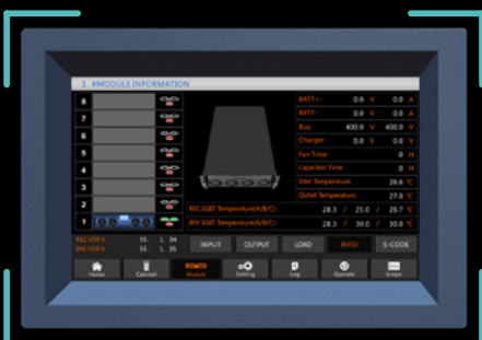
Information screen on the status of the power modules.
