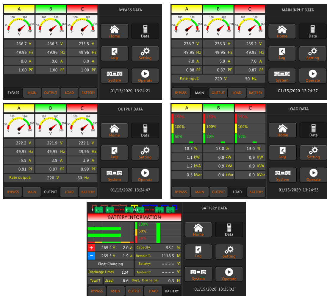
Figure 3-2 Submenu Interface of Data Page
